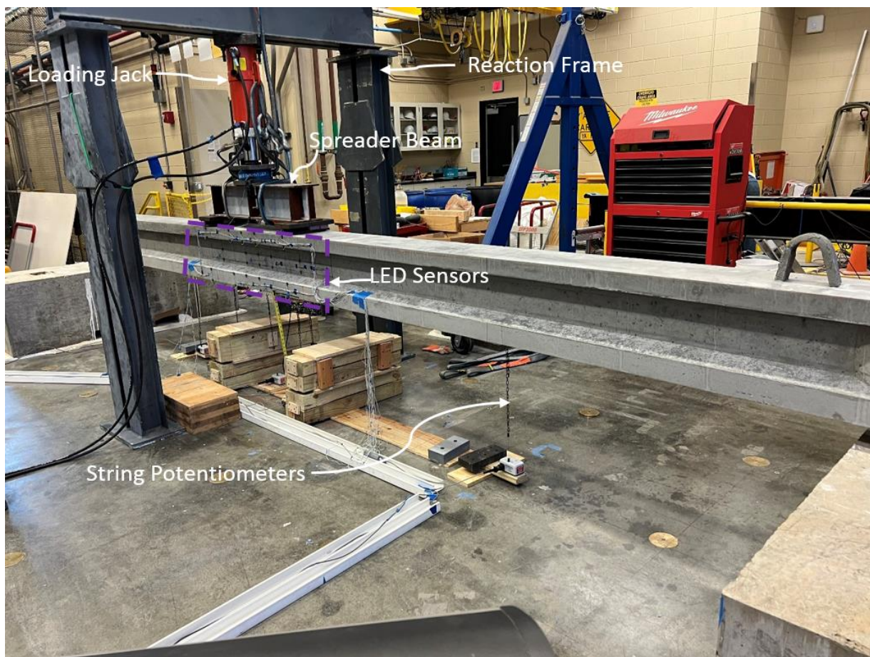
Figure 2: Test Setup of Big Beam
